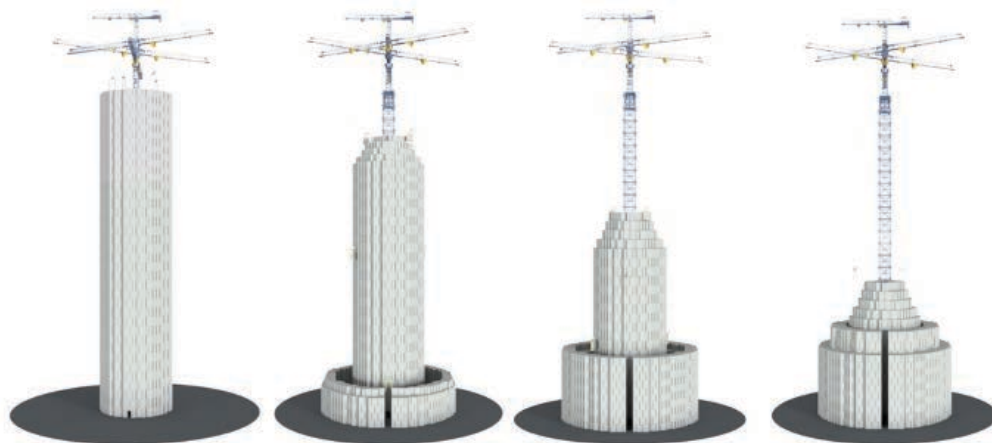
Figure 3.4 A model of the Energy Vault technology
