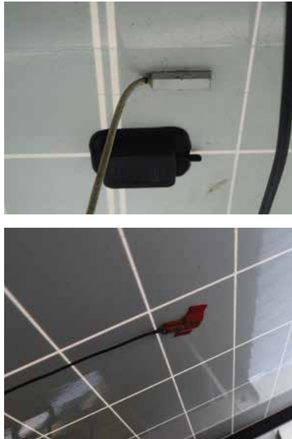
FIGURE 9.4 Examples of module temperature probes
