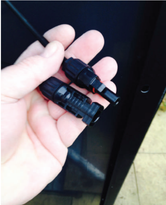
Figure 7.24 DC panel connections
