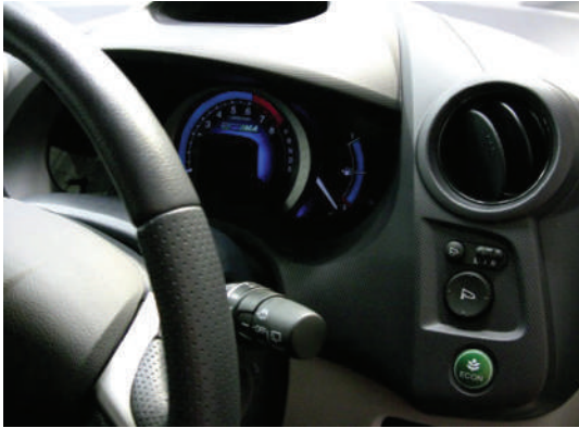
Figure 9.65 Feedback on economy/performance helps to change driving style and improve efficiency even more
