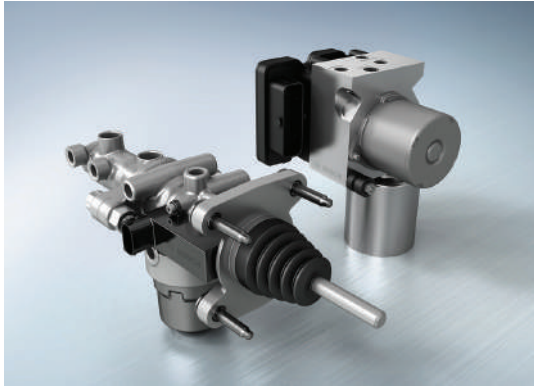
Figure 4.40 Vacuum-independent braking system specially designed for plug-in hybrids and electric vehicles. It comprises a brake operation unit (left) and an actuation control module (right) which supplement the ESP® hydraulic modulator (Source: Bosch Media)
