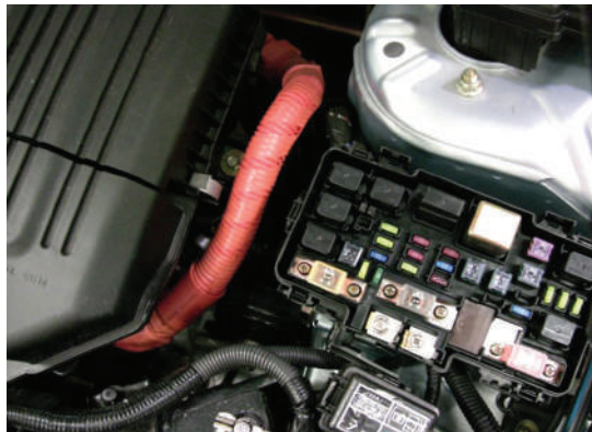
Figure 9.49 Power cable connected to the motor (remember, orange cables are high voltage)
