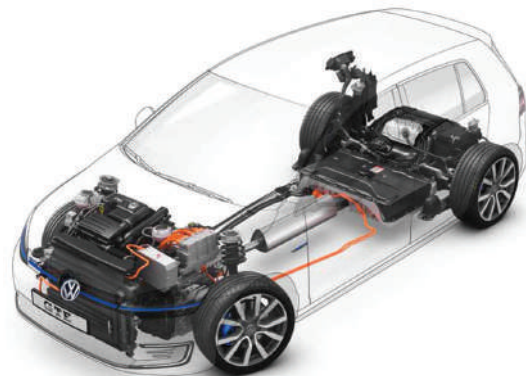
Figure 9.72 Golf GTE main components (Source: Volkswagen Media)
