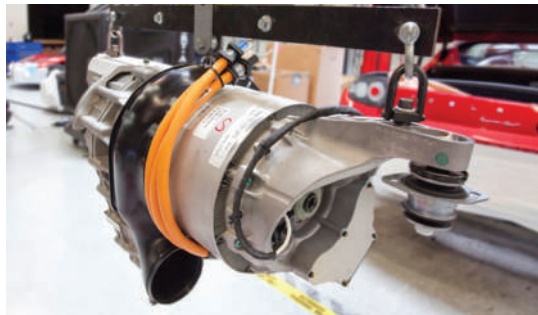
Figure 9.12 Tesla's AC induction motor (Source: Tesla Motors)
