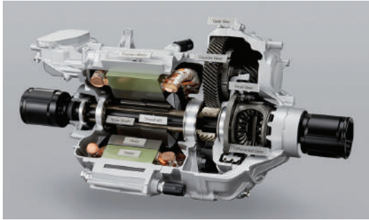
Figure 9.31 Induction drive motor, differential and final drive components (Source: Honda Media)
