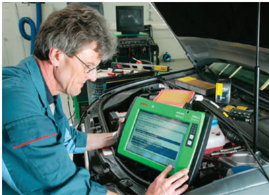
Figure 2.28 Diagnostic system in use (Source: Bosch Media)
