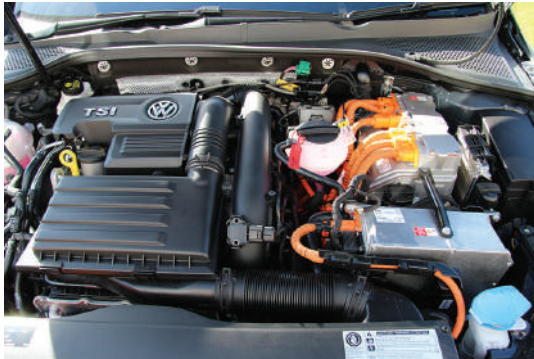
Figure 8.12 Golf GTE engine bay
