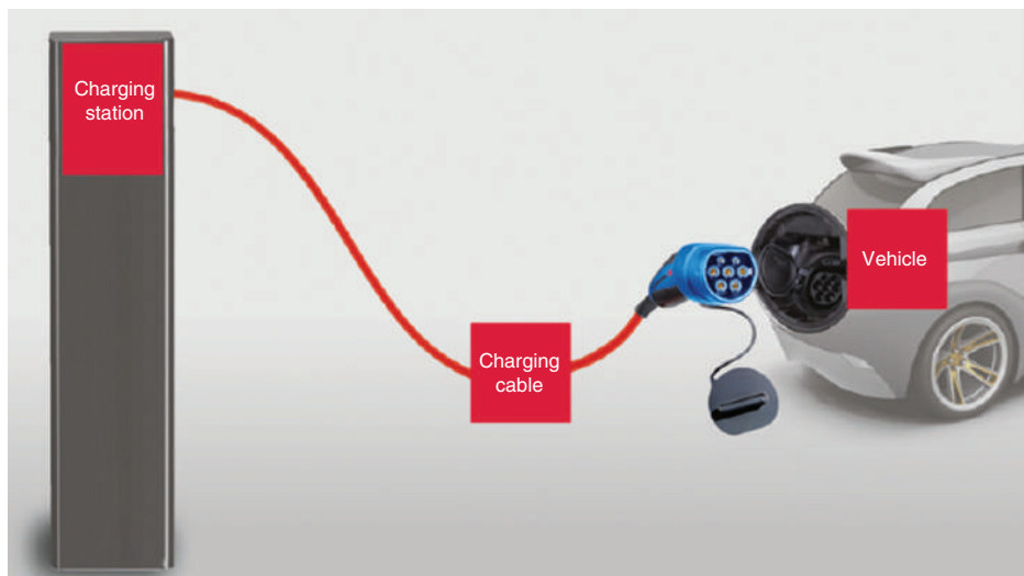
Figure 7.7 Case C: The charging cable is permanently connected to the charging station (Source: Mennekes)
